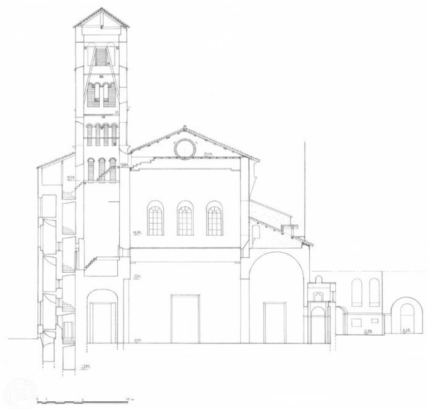
Fig. 433: Rome, S. Maria in Trastevere, transverse section through campanile and baptistery (Fulloni 1985/2016)
